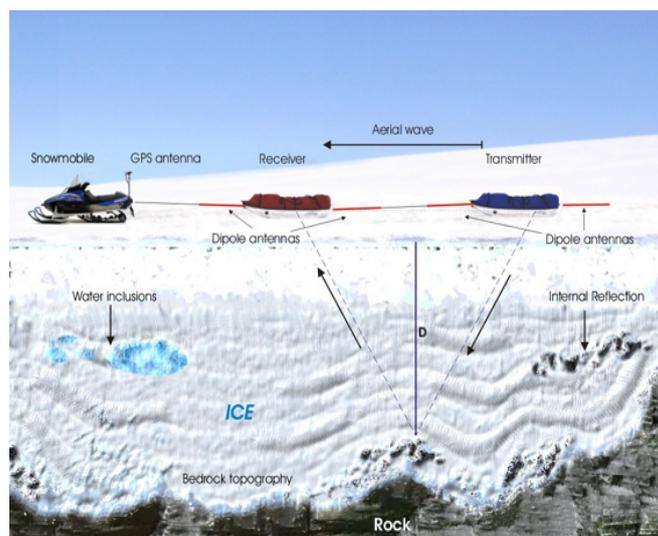
**Fig. 3.** Set of snowmobile, sleds, transmitter and receiver.
